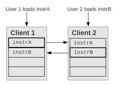
Figure 2: Instrument synchronization
